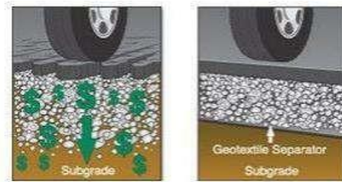
Figure 2.13 Geotextile for Separator
